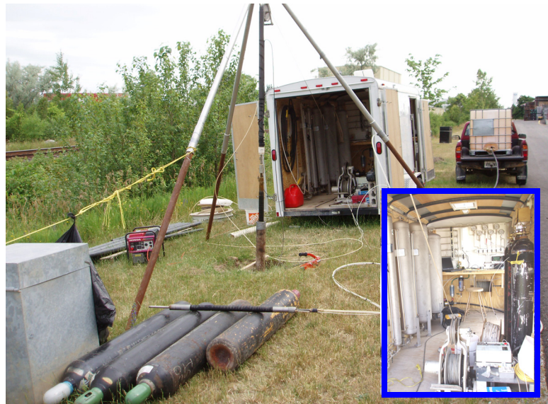
Fig. 8. A 3.78” straddle packer measurement system.
