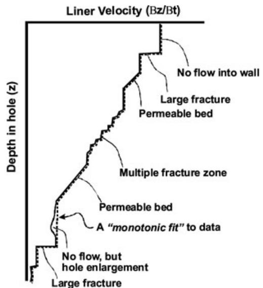
**Figure 4.** Hypothetical ideal “liner descent velocity profile” showing changes caused by several types of borehole features. The monotonic fitted line ignores temporary drops in liner velocity such as caused by a borehole enlargement where the liner velocity decreased but then increased upon exiting the enlargement.
