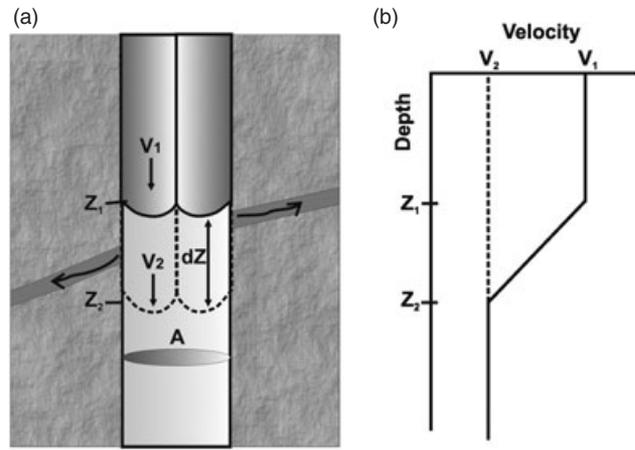
Flow rate into the fracture,  $\Delta Q = A(V_1 - V_2)$ , where  $V_1 > V_2$
