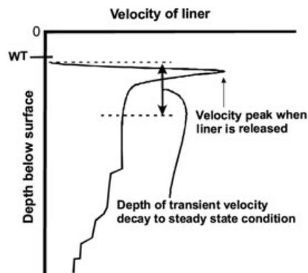
**Figure 6. Transient velocity decay to steady-state conditions during early stage of liner eversion.** Upon release of the liner, the liner velocity immediately peaks and then drops to the nominal steady-state flow rate. Thereafter, the velocity changes are governed by the sealing of transmissive features.
