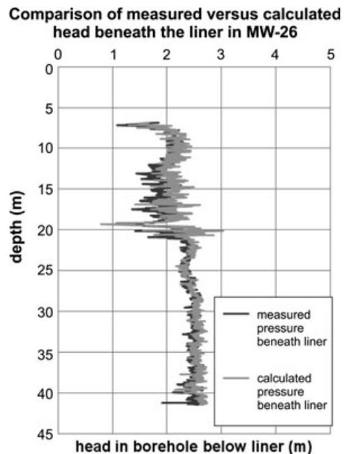
**Figure 8. Comparison of measured pressure history from the transducer at the bottom of the hole beneath the liner with the calculated pressure history using the measurements of the liner at the surface for MW-26. In this case, the agreement is very good and the transmissivity results are essentially the same using either history for this borehole. Boreholes with higher vertical flow rates (>38 L/min [10 gpm]) generally do not show such good agreement.**
