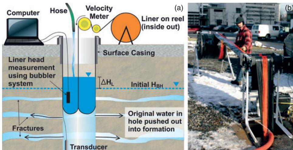
**Figure 2.** System components for the profiling method (a) (not to scale, vertically compressed). As water is added to maintain a constant head differential ( $\Delta H_L$ ) between inside the liner and the initial blended head, the liner descent rate (velocity) is measured as the head below the liner is measured (by the transducer) and (b) photograph showing the liner deployed from the shipping reel in the background and extending through the profiler positioned above the hole (foreground).
