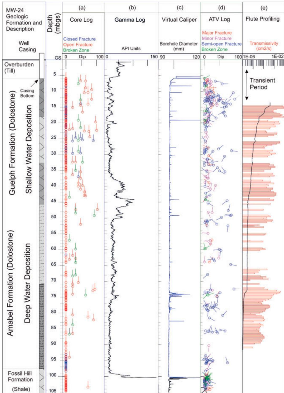
**Figure 10.** Geological and geophysical features in MW-24 displayed along the liner *T* profile. The core log, caliper, and ATV logs all indicate the presence of numerous fractures, which is consistent with the liner profile where the *T* values are integrated over 1-foot intervals.
