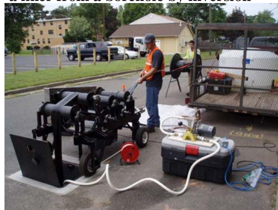
Fig. 4. FLUTE Linear Capstan removing a liner from a borehole by inversion
