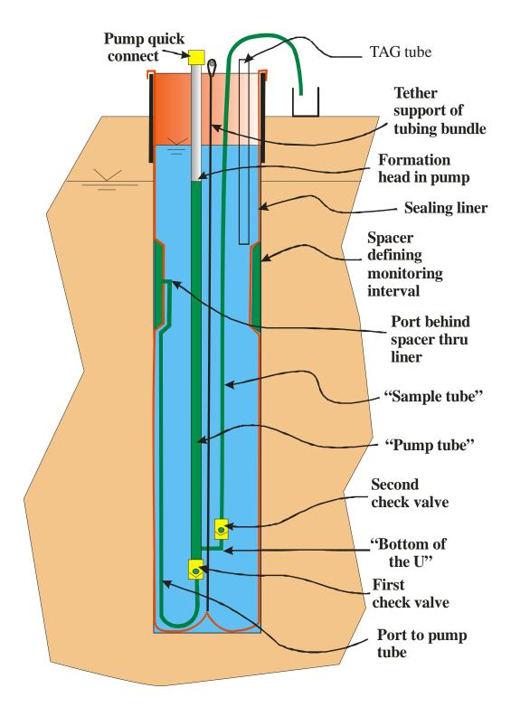
Fig. 2. Pumping Procedure
