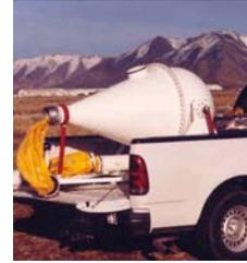
The Vadose FLUTE liner is made of a rugged Nylon fabric with an impermeable polyurethane coating. The tubing in the liner is gathered in sleeves welded to the inside surface of the liner. Exterior permeable spacers over each port are welded to the liner to allow sampling from an area, rather than from a spot, on the hole wall.
