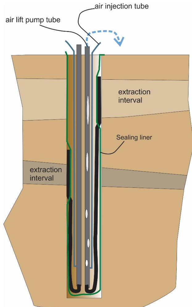
**Figure 1. The DEIL geometry showing the large tube from the extraction interval and the larger air lift pump tube. Air injected near the bottom of the pump tube reduces the density of the water column and causes it to be driven to the surface. Water table depth at the port should be less than half the liner depth.**
